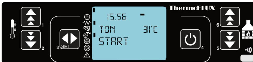
**START** will be displayed, on the left side of display we see that igniter and suction fan are activated. Mark **TON** is showing that room thermostat is connected or overbridged on connection for room thermostat (default). After that, on display we have text **LOAD PELLE** and on the left side we see that feeding of pellet is activ.
