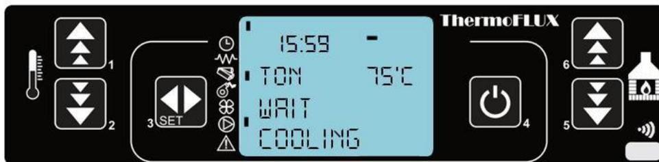
When temperature in the boiler decreases for 2 °C below set temp. regulation will start process of ignition again.
