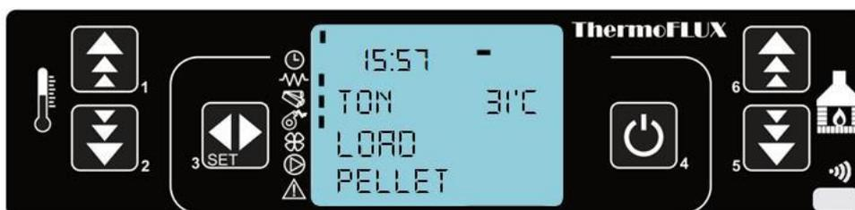
After ignition of pellet, and after temperature of flue gasses raise on value of 50°C, regulation receives signal that fire is on and boiler continues to work with set values.
